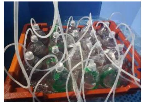
FIGURE 35 : PHOTO DE L'INSTALLATION POUR LA PRODUCTION DES LIXIVIATS A PARTIR DES ECHANTILLONS
